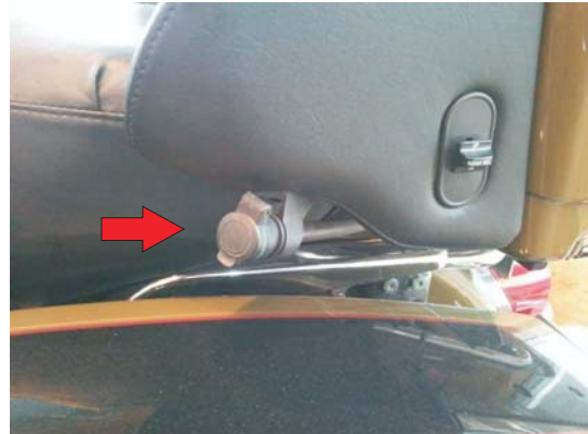
When driving solo, you can also use the back side plug for driver
