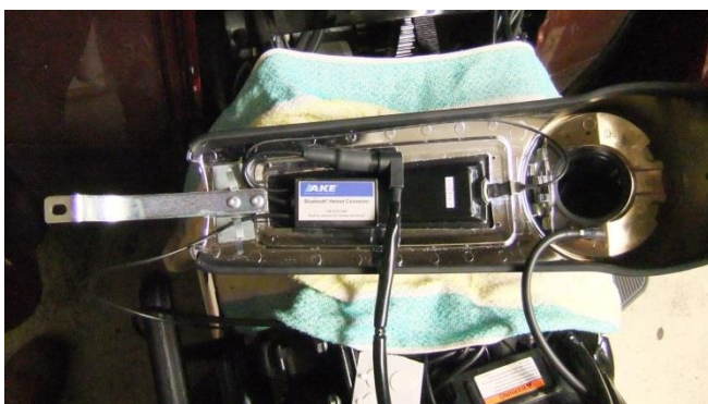
Reconnect all connectors and arrange the Box
