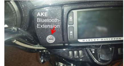
Built into the front panel instead of the helmet jack of the audio system
