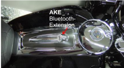
Built in the tank cover instead of the helmet jack for the driver
